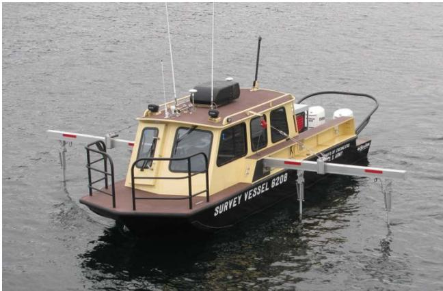
Now you can run sweep surveys with up to 24 channels in waters too shallow for practical multi beam survey with the Model 4810 Sweep System from Ross Laboratories! When connected to your PC running survey software, along with DGPS and heading sensor, you are ready to go!
